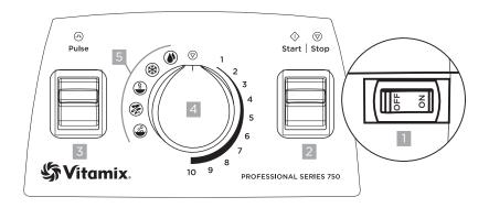
1. On / Off Switch: The On / Off (or Power) Switch is located on the lower right-hand side of the machine. The On / Off Switch controls the power to the machine.
